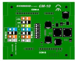
VCC - +12VDC GND - Masse/Ground
