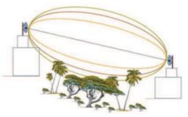
The diameter of the Fresnel zone determines how far above the ground and other obstacles the antennas must be. The diameter of the Fresnel zone depends on the frequency and the distances between the two transmitters.
