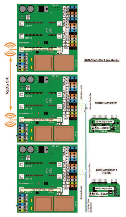
Terminal plan RF module with sub-communication to other controllers
