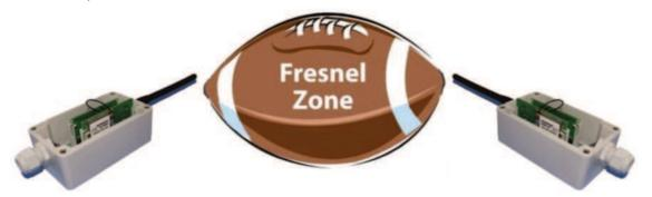
To achieve the greatest range, the Fresnel zone in which the radio waves travel must be free of obstacles. Buildings, trees or other obstacles in the way reduce the communication area.
