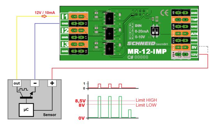
The additional analog input AIN can be configured as a 0-10V/0-20mA or as a digital input using a dip switch. Another PT1000 sensor input is also available.
