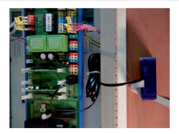
On controllers of the series 1.x (T-Print) the additional interface adapter has to be connected to the four-bus-terminals and then connect the flat cable there. cConnection diagram:
